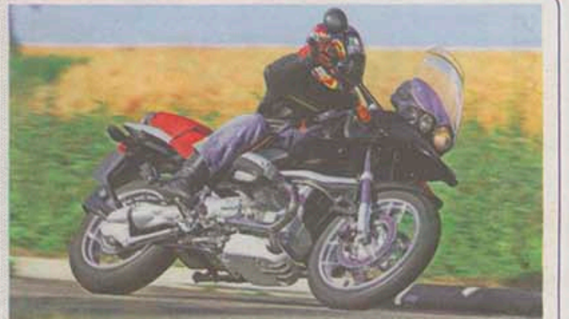
1994 R1100GS is launched and it not only gets a capacity hike, but it has the first four valve head boxer engine. Telelever front suspension system, featuring a wishbone and single shock, is added.
