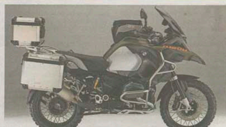
2013 All-new water-cooled engine sees power climb to 125bhp and there are a plethora of
